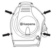
Loosen the two fasteners holding the air filter cowling and remove the filter. Wash the filter clean in warm, soapy water.
